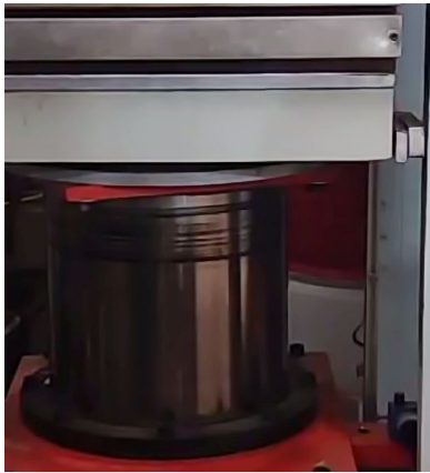
图4 GFRL/Mg 热模压固化设备 Fig.4 Hot molded curing equipment for GFRL/Mg
